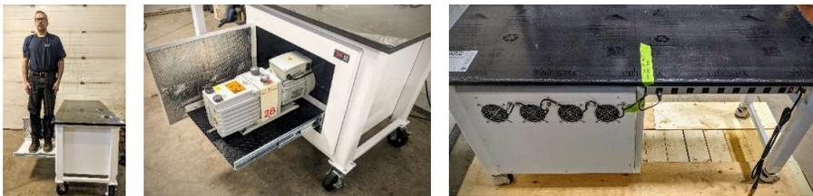
Sound dampening cabinet with 400 pound rated shelf. Will fit TWO E2M28 pumps or MS40+ pump with ease. Built in fans, digital temperature display with high temperature alarm. Default hose/electrical entrance is left and right side. Option for top holes (through benchtop).
