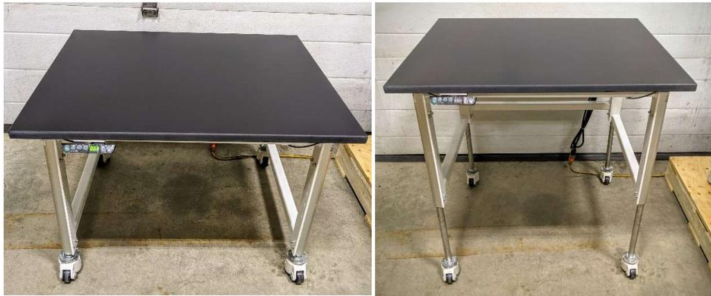
Electric-hydraulic lift table/workstation; 1000 pound (450 kg) capacity; 12 inch (30 cm) range
